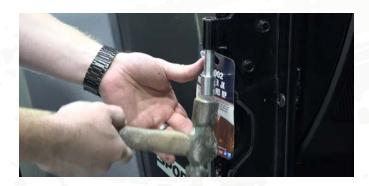
Using a hammer, tap the removal tool until the OE liner has been completely removed. You may need to tap the tool back though the hinge to remove it depending on how much corrosion has built up in the OE hinge. Repeat for all door hinges.
