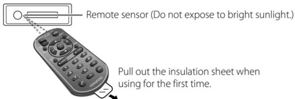
**KDC-X704 / KDC-X304 / KDC-BT778HD / KDC-BT378U / KDC-BT34** : Can be remotely controlled with an optionally purchased remote control.
