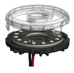
3. Release and remove lens
