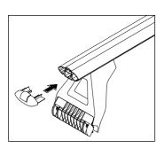
When the leg assemblies are fitted to the vehicle, then tighten M6 bolts to 3-4Nm. **Do not over tighten.** Measure slot length (A) and (B). Cut a piece of the underside strip and locate into the slots.
