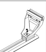
Insert the rubber buffer strip fully into the crossbar. Check the rubber buffer strip is fully inserted.
