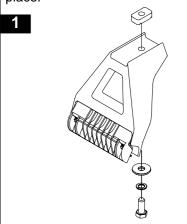
ASSEMBLY A1: Assemble M6 x 45mm, M6 spring washer, M6 square washer, leg height spacer block, adaptor block and M6 square nut as shown. ASSEMBLY A2: Assemble M6 x 55mm bolt, M6 spring washer, M6 square washer, the two leg height spacer blocks, adaptor block and M6 square nut as shown.
