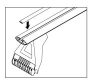
Insert the end cap completely into the crossbar.
