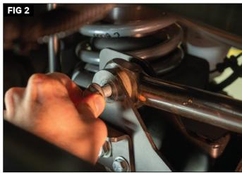
Put on safety glasses. Park the vehicle on a level surface. Set the parking brake and chock the wheels. Find the lower bolt that attaches the trackbar to the axle. Using a 21mm socket and rachet and wrench, remove this bolt. (Fig. 1) There is a flag bolt on the backside. of the bracket. Retain this hardware for reattaching the Lynx trackbar. (Fig. 2)
