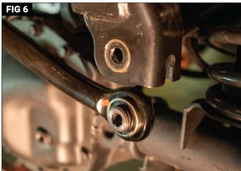
Retain the hardware for later use. (Fig. 5) Using both hands, carefully lift trackbar and remove from vehicle. (Fig. 5)
