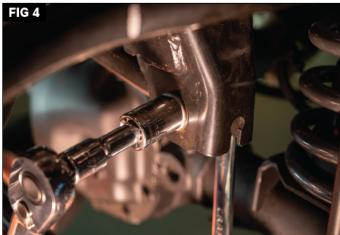
Locate the bolt holding the original trackbar to the frame. (Fig. 3) Remove using a 21mm socket with extension and rachet on one side and 21mm wrench on the other. (Fig. 4)
