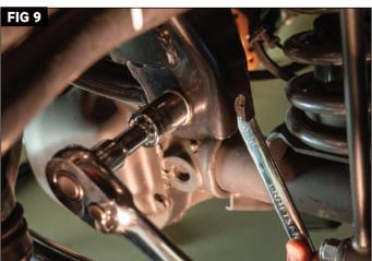
Using the hardware from Step 3, attach the non-adjustable end of the Lynx trackbar to the frame mount. (Fig. 8) Tighten but don't fully torque at this time. (Fig. 9)
