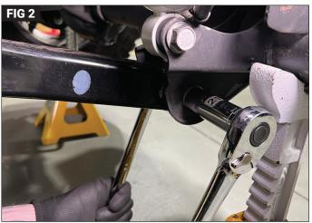
Put on safety glasses. Park the vehicle on a level surface. Set the parking brake and chock the wheels. Use jack stands and remove the wheels for easier access. Locate the bolts at each end on the lower control arms. (Fig.1) Using two 21mm wrenches or combination of 21mm socket and ratchet and wrench, remove each bolt and carefully remove the control arm. (Fig.2) Retain factory bolts, nuts and flag nuts for reuse.
