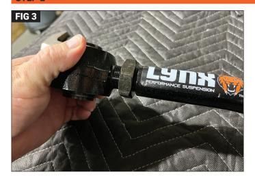
Set the Lynx Adjustable Control Arms to the factory length of 22 7/8" or to the desirable length based on your lift height. We recommend that you preset the length of the lower control arms. The length is measured from the center of the bushing to the center of the bushing at the other end. This length is a good starting point when using the stock length upper control arms, the final length should be adjusted by a professional to get the correct amount of castor, usually 4-6 degrees.
