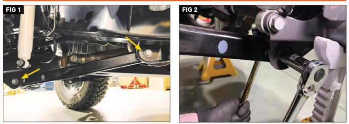
Put on safety glasses. Park the vehicle on a level surface. Set the parking brake and chock the wheels. Use jack stands and remove the wheels for easier access. Locate the bolts at each end on the lower control arms. (Fig.1) Using two 21mm wrenches or combination of 21mm socket and ratchet and wrench, remove each bolt and carefully remove the control arm. (Fig.2) Retain factory bolts, nuts and flag nuts for reuse.
