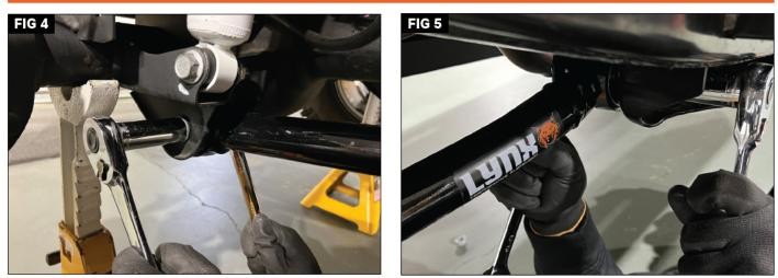
Install the new control arms with the bushing at the axle mount (Fig. 4) and the adjustable point at the frame mount (Fig. 5). Reuse the factory mounting bolts from Step 1. Tighten the factory control arm bolts to 125 ft-lbs, wait until the vehicle is at ride height before tightening the rubber bushing end. Once final length adjustments are made, tighten the jam nut bolt to 80 ft-lbs. Repeat steps for opposite side of vehicle.
