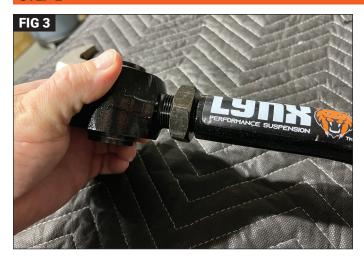
Set the Lynx Adjustable Control Arms to the factory length of 19 3/4" or to the desirable length based on your lift height. We recommend that you preset the length of the lower control arms. The length is measured from the center of the bushing to the center of the bushing at the other end. The final length should be adjusted by a professional to get the correct amount of castor with an alignment.
