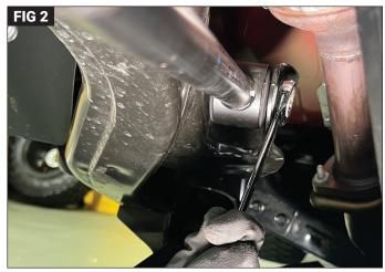
Put on safety glasses. Park the vehicle on a level surface. Set the parking brake and chock the wheels. Use jack stands and remove the wheels for easier access. Locate the bolts at each end on the upper control arms. Using two 21mm wrenches or combination of 21mm socket and ratchet and wrench, remove each bolt and carefully remove the control arm. (Fig. 1 & 2) Retain factory bolts, nuts and flag nuts for reuse.
