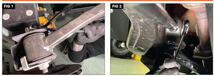
Put on safety glasses. Park the vehicle on a level surface. Set the parking brake and chock the wheels. Use jack stands and remove the wheels for easier access. Locate the bolts at each end on the upper control arms. Using two 21mm wrenches or combination of 21mm socket and ratchet and wrench, remove each bolt and carefully remove the control arm. (Fig. 1 & 2) Retain factory bolts, nuts and flag nuts for reuse.
