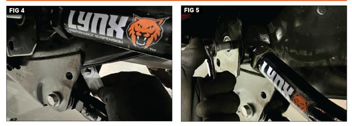
The flag bolt for the upper frame mount should be carefully placed up and through the frame cutout. (Fig. 4) Attach the adjustable point at the frame mount using the factory bolt from Step 1 (Fig. 5). Once the vehicle is on the ground and at ride height, tighten the factory control arm bolts to 125 ft-lbs. Once final length adjustments are made, tighten the jam nut bolt to 80 ft-lbs. Repeat steps for opposite side of vehicle.
