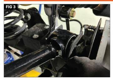
Set the Lynx Adjustable Control Arms to the factory length of 17 1/4" or to the desirable length based on your lift height. We recommend that you preset the length of the lower control arms. The length is measured from the center of the bushing to the center of the bushing at the other end. The final length should be adjusted by a professional to get the correct amount of castor with an alignment.
