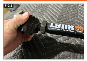
Set the Lynx Adjustable Control Arms to the factory length or to the desirable length based on your lift height. We recommend that you preset the length of the lower control arms. The length is measured from the center of the bushing to the center of the bushing at the other end. This length is a good starting point when using the stock length upper control arms, the final length should be adjusted by a professional to get the correct amount of castor, usually 4-6 degrees.
