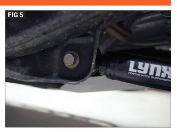
Install the new control arms with the bushing at the axle mount (Fig. 4) and the adjustable point at the frame mount (Fig. 5). Reuse the factory mounting bolts from Step 1. Re-attach the brake line bracket. Tighten the factory control arm bolts to 125 ft-lbs, wait until the vehicle is at ride height before tightening the rubber bushing end. Once final length adjustments are made, tighten the jam nut bolt to 80 ft-lbs. Repeat steps for opposite side of vehicle.
