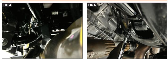
Install the new control arms beginning at the axle mount (Fig. 4) and then the adjustable point at the frame mount (Fig. 5). Reuse the factory mounting bolts from Step 1. Tighten the factory control arm bolts to 125 ft-lbs., wait until the vehicle is at ride height before tightening the rubber bushing end. Once final length adjustments are made, tighten the jam nut bolt to 80 ft-lbs. Replace the shielding with the two 10mm bolts. Repeat steps for opposite side of vehicle.
