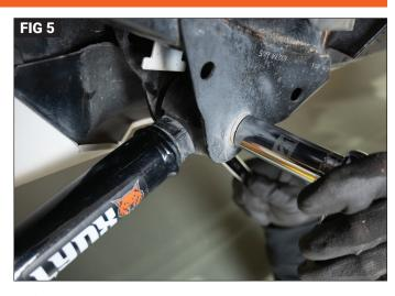
Install the new control arms with the bushing at the axle mount (Fig. 4) and the adjustable point at the frame mount (Fig. 5). Reuse the factory mounting bolts from Step 1. Tighten the factory control arm bolts to 125 ft-lbs., wait until the vehicle is at ride height before tightening the rubber bushing end. Once final length adjustments are made, tighten the jam nut bolt to 80 ft-lbs. Repeat steps for opposite side of vehicle.
