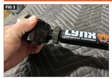
Set the Lynx Adjustable Control Arms to the factory length or to the desirable length based on your lift height. We recommend that you preset the length of the lower control arms. The length is measured from the center of the bushing to the center of the bushing at the other end. The final length should be adjusted by a professional to get the correct amount of castor with an alignment.
