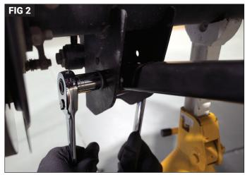
Put on safety glasses. Park the vehicle on a level surface. Set the parking brake and chock the wheels. Use jack stands and remove the wheels for easier access. Locate the bolts at each end on the lower control arms. (Fig.1) Using a 21mm wrenches or 21mm socket and ratchet and wrench, remove each bolt and carefully remove the control arm. (Fig.2) Retain factory bolts, nuts and flag nuts for reuse.
