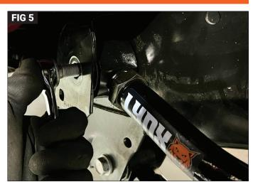
The flag bolt for the upper frame mount should be carefully placed up and through the frame cutout. (Fig. 4) Attach the adjustable point at the frame mount using the factory bolt from Step 1 (Fig. 5). Once the vehicle is on the ground and at ride height, tighten the factory control arm bolts to 125 ft-lbs. Once final length adjustments are made, tighten the jam nut bolt to 80 ft-lbs. Repeat steps for opposite side of vehicle.
