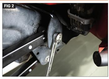
Put on safety glasses. Park the vehicle on a level surface. Set the parking brake and chock the wheels. Use jack stands and remove the wheels for easier access. Locate the bolts at each end on the upper control arms. Using two 21mm wrenches or combination of 21mm socket and ratchet and wrench, remove each bolt and carefully remove the control arm. (Fig. 1 & 2) Retain factory bolts, nuts and flag nuts for reuse.
