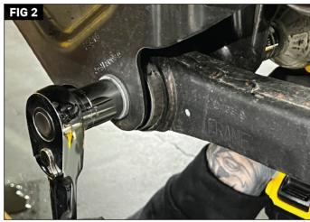
Put on safety glasses. Park the vehicle on a level surface. Set the parking brake and chock the wheels. Use jack stands and remove the wheels for easier access. Locate the bolts at each end on the lower control arms. (Fig.1) Using a 21mm wrenches or 21mm socket and ratchet and wrench, remove each bolt and carefully remove the control arm. (Fig.2 & 3) Retain factory bolts nuts for reuse.
