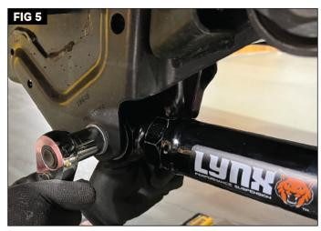
Install the new control arms with the bushing at the axle mount (Fig. 4) and the adjustable point at the frame mount (Fig. 5). Reuse the factory mounting bolts from Step 1. Tighten the factory control arm bolts to 125 ft-lbs., wait until the vehicle is at ride height before tightening the rubber bushing end. Once final length adjustments are made, tighten the jam nut bolt to 80 ft-lbs. Repeat steps for opposite side of vehicle.
