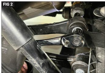
Put on safety glasses. Park the vehicle on a level surface. Set the parking brake and chock the wheels. Use jack stands and remove the wheels for easier access. Locate the bolts at each end on the upper control arms. (Fig. 1) Using two 21mm wrenches or combination of 21mm socket and ratchet and wrench, remove each bolt and carefully remove the control arm. (Fig. 2 & 3) Retain factory bolts nuts for reuse.
