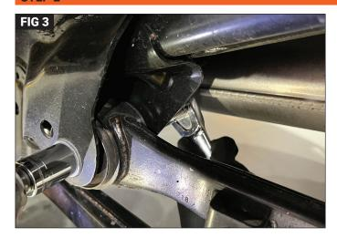
Set the Lynx Adjustable Control Arms to the factory length or to the desirable length based on your lift height. We recommend that you preset the length of the upper control arms. The length is measured from the center of the bushing to the center of the bushing at the other end. The final length should be adjusted by a professional to get the correct length with an alignment.
