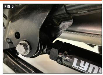
Install the new control arms with the bushing at the axle mount. (Fig. 4) Attach the adjustable point at the frame mount using the factory bolt from Step 1 (Fig. 5). Once the vehicle is on the ground and at ride height, tighten the factory control arm bolts to 125 ft-lbs. Once final length adjustments are made, tighten the jam nut bolt to 80 ft-lbs. Repeat steps for opposite side of vehicle.
