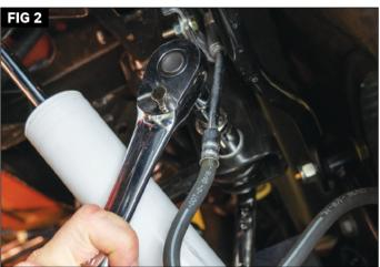
Put on safety glasses. Park the vehicle on a level surface. Set the parking brake and chock the wheels. Locate the bolt holding the original trackbar to the frame. (Fig. 1) Remove using a 21mm socket with extension and rachet on one side and 21mm wrench on the other. (Fig. 2) Retain the hardware for later use.
