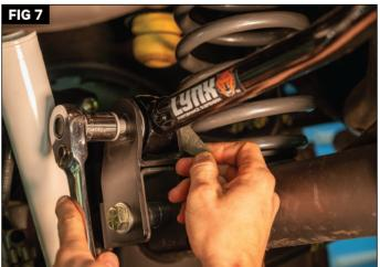
Using the hardware from Step 2, attach the non-adjustable end of the Lynx trackbar to the axle mount. (Fig. 6) Tighten but don't fully torque at this time. (Fig. 7)
