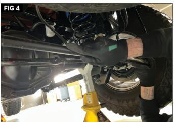
Find the lower bolt that attaches the trackbar to the axle. Using a 21mm socket and rachet and wrench, remove this bolt. There is a flag bolt on the backside of the bracket. (Fig. 3) Retain this hardware for reattaching the Lynx trackbar. Using both hands, carefully lift trackbar and remove from vehicle. (Fig. 4)
