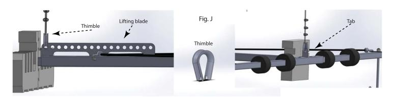
As shown in Fig. K, feed the cable through the hole with the thimble, install cable clamps loosely at first, in order to balance the frame. With the frame level on the floor pull the cable taut and secure the cable clamps in the order shown in figure K. Be careful to not over tighten these as they will strip. If they do become stripped or are suspect do not use them, they can be inexpensively obtained at any hardware store. Inspect these and all hardware before each use.
