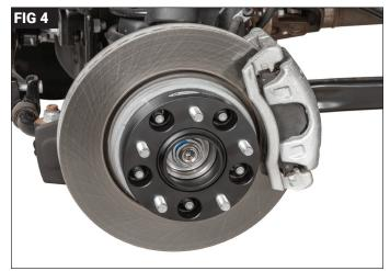
Apply the provided thread locker to the original wheel studs as shown. (FIG 3) Slide the Wheel Spacer and/or Adapter onto the wheel studs as shown. (FIG 4)
