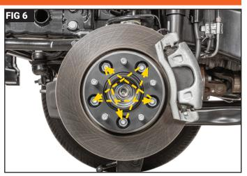
Install the supplied Wheel Spacer and/or Adapter Lug Nuts as shown with the tapered seat facing inward. Thread the Lug Nuts on as much as possible finger tight in a star pattern. (FIG 5) **NOTE:** Do not use an Impact Gun. With the help of a friend, apply the brakes to keep the drum/rotor from spinning, and begin to tighten the Lug Nuts per the vehicle's owner manual specifications in a star pattern as shown. (FIG 6)
