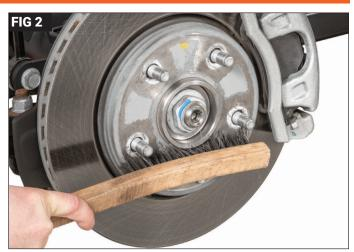
If present, remove the brake drum or rotor disc retaining clips using a flat blade screwdriver and diagonal cutting pliers. (FIG 1) Thoroughly clean the wheel studs, hub area, and brake drum and/or rotor disc using a wire brush. (FIG 2)
