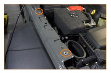
08. Install 2x fender brackets for the snorkel (4x 25mm M6 hex head bolts, 4x M6 flat washers). **DO NOT FULLY TIGHTEN THE BOLTS**.
