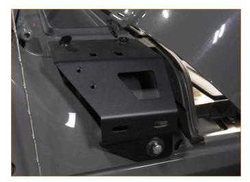
Install the smallest bracket onto the large bracket (2x 14mm M6 bolts, 2x M6 flat washers, 2x bolt caps). DO NOT FULLY TIGHTEN THESE BOLTS.
