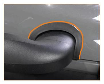
23. Now remove the bezel, apply silicone sealant (not included) inside and secure it to the hood matching the outline you marked in the previous step. This is to ensure proper alignment of the bezel when opening and closing the hood.
