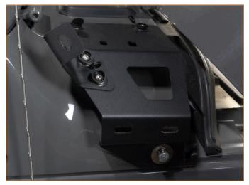
Install the main snorkel tube. Connect the intake end of the snorkel tube with the rubber air duct and ensure it is fully seated. Attach snorkel to the first bracket installed on the fender (2x 14mm M6 bolts, 2x M6 flat washers, 2x bolt caps).
