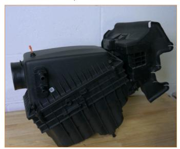
**03.** Remove the upper airbox lid and panel filter, then remove stock air duct from the lower airbox.
