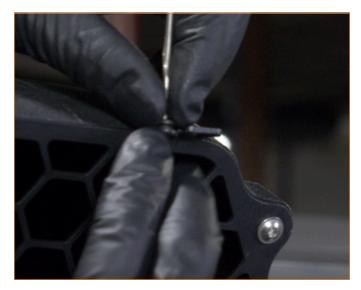
**21.** Install the rubber hood bezel temporarily. It should be able to move along the cutout on the hood.
