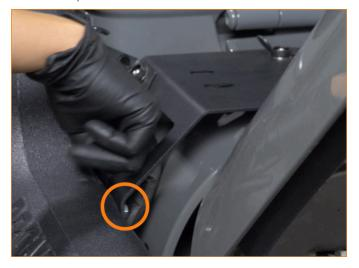
Attach the snorkel to the second bracket installed on the fender with 2x M4 button head flanged bolts. DO NOT FULLY TIGHTEN THESE BOLTS.
