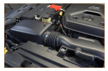
07. Remove 2x 10mm hex head bolts on the passenger side fender.
