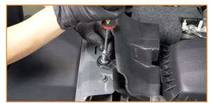
6. Separate the two quick-disconnect fittings from the airbox.
