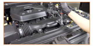
2. Loosen the clamps on each end of the intake tube, where it connects to the airbox and intake muffler. (2x worm gear clamps)
