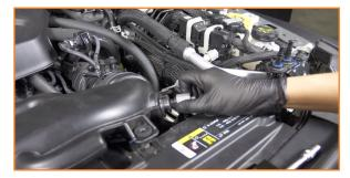
4. Slide off the intake tube from its connections and lift it out of the vehicle.
