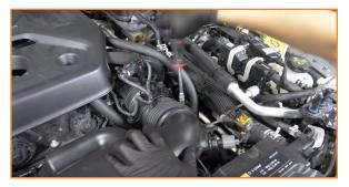
3. Disconnect the air temp sensor and release the wiring harness. (1x tree-clip)
