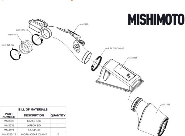
Below is an exploded diagram of the Mishimoto intake and all the parts included for reference during installation.
