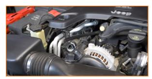
2. Disconnect the intake air temperature sensor from the intake tube. Release its wiring harness. One clip is linked to a nearby coolant hose. (3x tree-clips)
