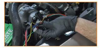
28. Cut the bullet connectors off the blue wire coming from each fan. Twist the two cut wires together. Put them inside the male spade connector and crimp the connector. Apply solder to the assembly.
