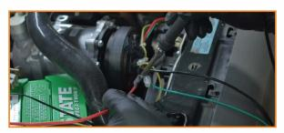
33. Run the black wire from the fan controller to the battery's negative terminal. Repeat previous steps for attaching a connector to this wire—strip, crimp, solder, and seal the assembly.
