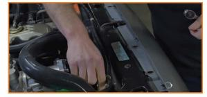
Detach the metal support just behind the grille's top edge. (4x 10mm bolts)
