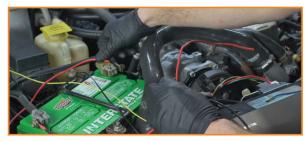
30. Strip both ends of the red wire. Crimp the shown connector onto one end. Apply solder and seal the connector using 1" of heat shrink.
