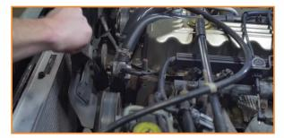
Remove the brackets that hold the AC condenser to the radiator. (2x 8mm nuts)
