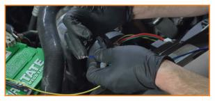
29. Run the provided red wire behind the battery to the positive terminal. The other end runs to the blue wire. Cut the excess wire.
