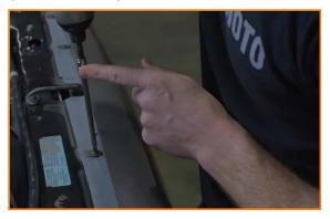
Remove the bolts that secure the upper support bar. You will need to remove the battery to reach one of the covered bolts. (6x 10mm bolts)
