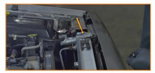
11. Put the push probe sensor about 3" down from the top of the radiator and 1" over from the header plate.
