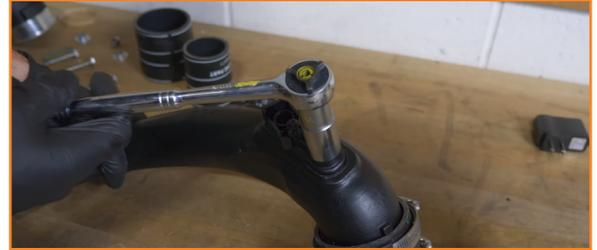
11. Install the MAP sensor onto the Mishimoto pipe.
