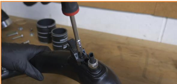
10. Remove the temperature sensor from the intercooler pipe. Then install it onto the Mishimoto pipe. Snug it down until tight.
