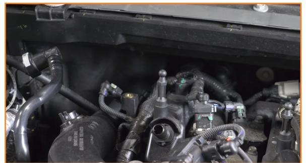
5. Disconnect the blow-off valve electrical harness. Lift the red tab and depress the black tab at the center to separate the connection.
