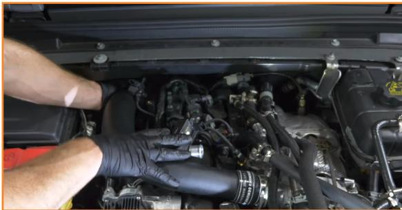
19. Slide the larger side over the throttle body. It may be necessary to angle the larger coupler on the intercooler pipe to get them to easily slide onto the throttle body.
