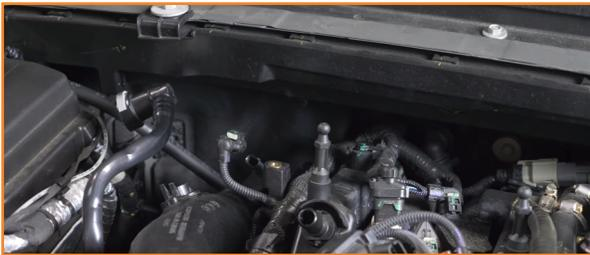
7. Loosen the clamps that hold the hoses on the intercooler pipe.
