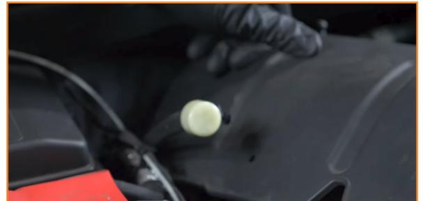
4. Disconnect the ventilation port for the valve cover. Pull the gray tab to free the connection.
