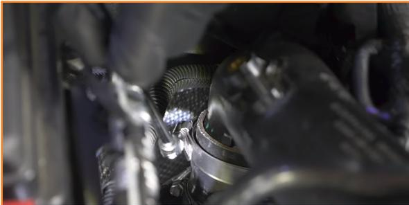
8. Remove the stock intercooler pipe.
