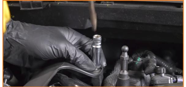
3. Release the breather attached to the heat shrouding. (2x pop-clips)
