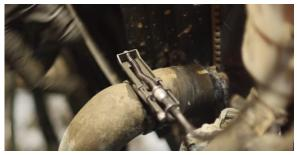
Disconnect the fan shroud's electrical harness.
