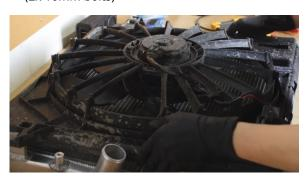
20. Transfer the overflow hose from the stock radiator to the Mishimoto radiator.(1x worm gear clamp, or 1x spring clamp)
