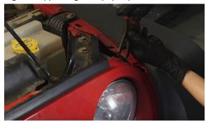
3. Disconnect the electrical harness located on the bottom of each side of the grille. To disconnect this harness, lift the red tab and then depress the black tab at the center.
