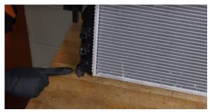
2. There are six clips that secure the top of the grille to the support bar. Pull these clips out to free the grille's upper edge. (6x pop-clips)
