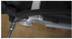
21. Transfer the rubber bushings on the stock radiator to the Mishimoto radiator's brackets.
