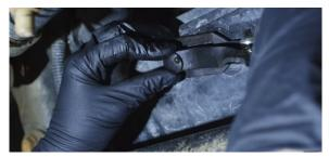
7. Loosen the clamp on the intake tube and airbox connection. (1x worm gear clamp)
