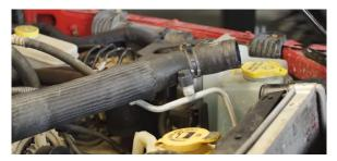
10. Compress the clamp on the lower radiator hose and slide it down the hose. Then pull the hose off the radiator port. (1x spring clamp)
