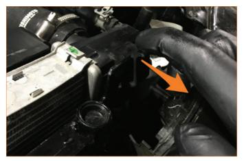
Remove the bolts that secure the horn brackets to the radiator support (2x 10mm bolts) and replace them with provided allen bolts (2x 4mm allen bolts).
