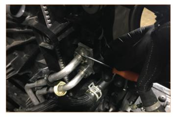
Remove the bolts securing the top of the radiator to the radiator support (2x 10mm bolts).
