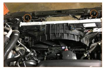
Transfer the quick-disconnect fittings from the stock transmission cooler to the Mishimoto transmission cooler (2x quick disconnect fittings)
