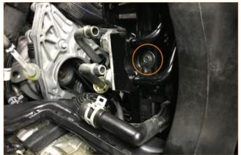
13. Pull back on the tab located on the driver side of the radiator that secures the transmission cooler to the radiator and remove the transmission cooler from the vehicle.
