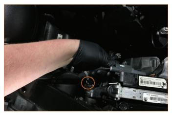
09. Remove the passenger-side headlight from the vehicle (3x 10mm bolts and 1x electrical harness connector).
