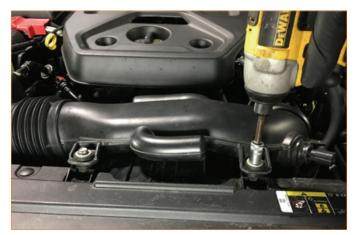
**06.** Remove the vacuum lines from the intake air box and then remove the air intake assembly from the vehicle. (2x vacuum lines)
