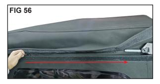
Locate the drivers rear quarter window. Line up the driver's side Quarter window to the zipper on the top deck and zip it as shown in FIG's 56 & 57
