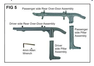
Locate the driver's side rear over door assembly, the driver's side Pillar assembly, the Rubber seal and the 4mm Allen head wrench (Fig 5).
