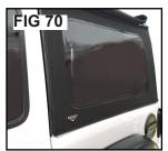
Note: You may have to pull the corners around towards the front or back of the vehicle to center the top on the vehicle. If this is too difficult, release the front windshield header latches. Once installed the first time these windows will easily install. Repeat this on the passenger side centering the top over the rear bow.
