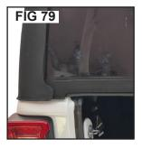
Take the tailgate bar and orient the "C"-Channel with the round seal facing down and slide the "C" Channel onto the rear window retainer as shown in FIG 74 & 75. After sliding the retainer all the way through the "C" Channel, roll the tailgate bar into the corner mounts with the outside of the fabric facing towards the rear of the Vehicle (Fig. 76).
