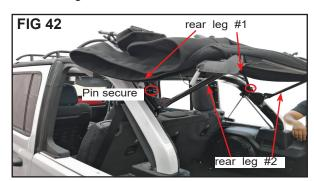
Step 12: Installing the top Deck
