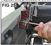
Step 8: Installing the rear bow #1 to the rear leg bracket
