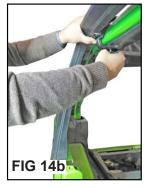
Locate the assembled Driver's side rear door surround previously installed in step 3.(Fig 9) and a set of screw knobs.
