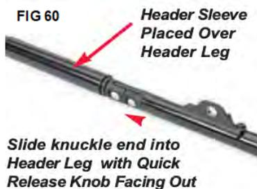
**Slide knuckle end into Header Leg with Quick Release Knob Facing Out**
