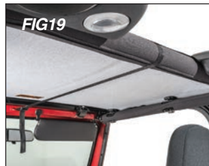
Bimini without Sound Bar: Simply wrap center strap around sport bar hoop.
