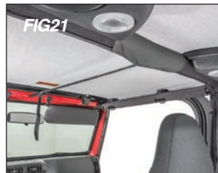
Bimini Plus without Sound Bar: Simply wrap center strap around sport bar hoop.
