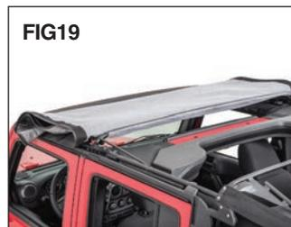
Un-latch the bow assembly from the windshield (inside vehicle) and lower the bow assembly to the rear of the vehicle folding the top back over with the underside of the fabric facing down (see FIG 19)
