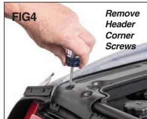
Make sure you keep all screws and fasteners in a safe place after removal. You will be using them again later in the installation. See FIGS 1, 2, 3 & 4
