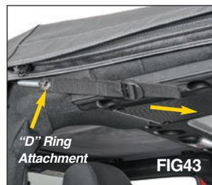
Please Note: If you fold down your front header and it is EXTREMELY TIGHT, STOP. To ensure the top fits properly you will need to un-screw the rear bow screws, fold down the header and then re-install the rear bow screws. This will prevent possible damage to the hardware system.
