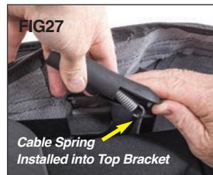
For 2013-2018 models the bracket is encased in a plastic "tube". As shown in FIGs 24-27, slip the cable spring through the "tube" and attach it to the top bracket and using a set of pliers, crimp the spring end closed so it cannot be easily slipped off.
