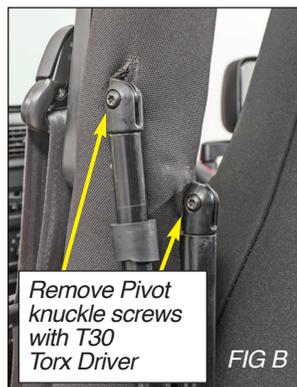
Remove Pivot knuckle screws with T30 Torx Driver
