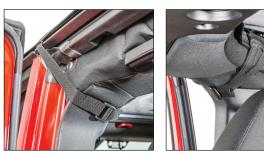
**Step 4** (4-Door) Install Side Tension Straps. Thread Side Tension straps through the buckle on side of the Bimini Plus. Hook end of the strap under the belt rail and slide it under the door surround. Pull the strap tight. Repeat on opposite side of vehicle.
