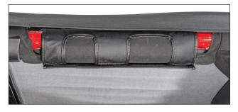
**Step 4** (for Bimini Plus 2-Door) Secure side straps onto Horizontal sport bars.
