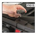
Locate the two sets of screw knobs. There should be (2) sets of three knobs with two the same length and one shorter length. The shorter knob attaches to the center hole on the door surrounds and the (2) longer knobs go on the front and rear holes.
