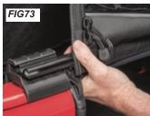
Open the tailgate. Take the factory tailgate bar and orient the "C"-Channel with the round seal facing down. Slide the "C" Channel onto the rear window retainer as shown in FIG's 70 & 71.
