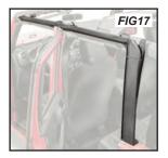
Finally, with the short knob, secure the "sandwiched" front & rear door surrounds (FIG 15) with the short knob and tighten all three knobs (FIGs 16 & 17). All knobs on both sides of the vehicle should be secured to the roll bar.
