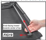
Locate the two quick release knobs and the Header/Deck Assembly with the over bow door attached as shown in FIG
