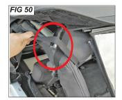
With the front header folded back towards the rear of the vehicle and on top of the second bow (FIG 46), locate the rear spring straps that is sewn on the rear end of the deck (FIG 47).
