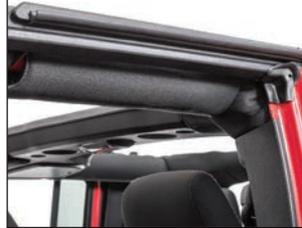
Work your way forwards towards the Front of the vehicle securing the extrusion along the way.
