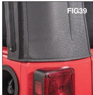
**Step 10: Attach Rear Corners into Body**
