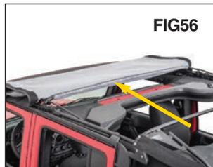
From inside the vehicle, attach the hook and loop flap around the front bow (Bow #1 over the sound Bar). See FIG 56.
