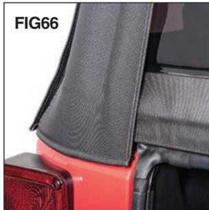
Tuck the flaps under the window zippers into the retainers to secure the rear window.
