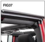
Work your way forwards towards the Front of the vehicle securing the extrusion along the way.
