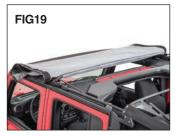
Un-latch the bow assembly from the windshield (inside vehicle) and lower the bow assembly to the rear of the vehicle folding the top back over with the underside of the fabric facing down (see FIG 19)
