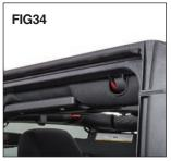
The soft lip should be facing up and the small plastic strip should fill in the gap on the door surround hardware. Work your way back towards the rear of the vehicle securing the extrusion along the way. Repeat the above for opposite side of top.
