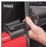
After sliding the retainer all the way through the "C" Channel, roll the tailgate bar into the mounts with the outside of the fabric facing towards the rear of the vehicle.
