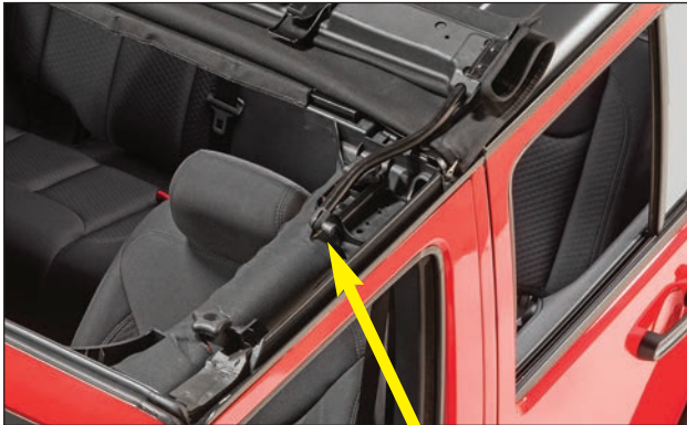
Brackets mounted on the Horizontal Roll Bar provide the pivot point for the SkyMaster fold back sun roof feature
