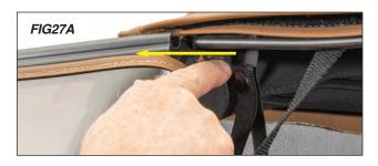
**Each Time you remove the rear window:** Completely pull the windows out of the "C" Channel before pulling the window down!
