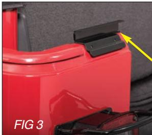
Hand tighten all provided #8 x 1/2" Pan Head washer screws into place holding the Tailgate bracket in place (Fig 3). Repeat on other side of Tailgate opening.
