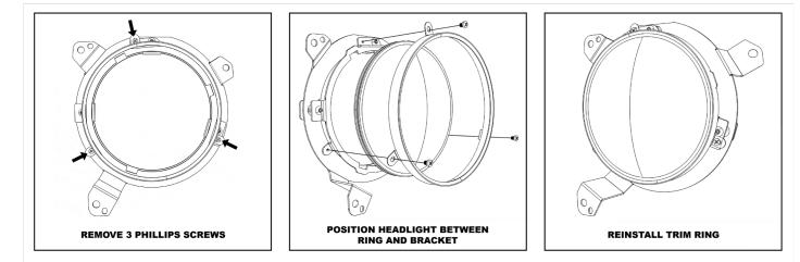
**4. Install the new LED headlights:** Now that the factory headlights are removed, it's time to install the XKGLOW headlights. Simply follow the instructions above but in reverse order. Plug the headlights in and secure them with the metal mounting rings. Pop the grill back into place and re-install the screws and pop clips.
