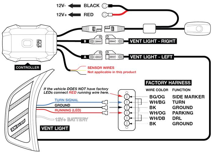
**5. Secure all wires and connectors:** Use provided screws or zip ties to neatly mount and hide any loose wires. The tabs can also be cut off to help the wire fit through tight spaces. Make sure they are not touching anything hot or located on moving parts. Install the ON/OFF switch in a dry and convenient location. Use provided end caps to cover all uncovered connectors.
