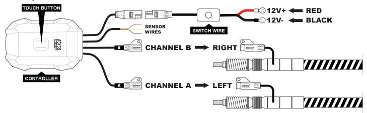
**2. Route wiring:** Secure XKmax Controller in a safe, accessible location. Plug in the 13ft extension wire and route it to the rear of the vehicle. Tip- using a zip tie, tie the wire off near where the mounting base will be located so that when the whip is not attached and plugged in, the plug will still stay near for next time it's needed.
