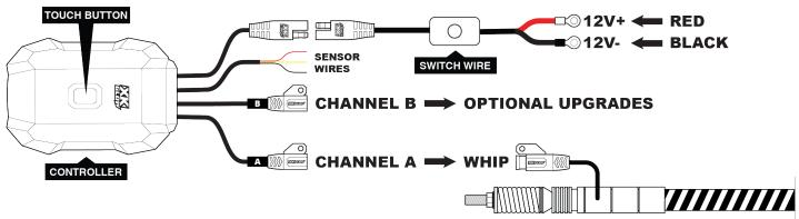
**2. Route wiring:** Secure XKmax Controller in a safe, accessible location. Plug in the 13ft extension wire and route it to the rear of the vehicle. Tip- using a zip tie, tie the wire off near where the mounting base will be located so that when the whip is not attached and plugged in, the plug will still stay near for next time it's needed.
