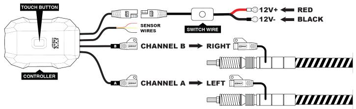
**2. Route wiring:** Secure XKmax Controller in a safe, accessible location. Plug in the 13ft extension wire and route it to the rear of the vehicle. Tip- using a zip tie, tie the wire off near where the mounting base will be located so that when the whip is not attached and plugged in, the plug will still stay near for next time it's needed.
