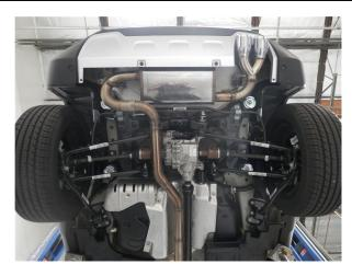
**Step 4.** Next using the supplied 2.50" clamp attach the Muffler Assembly to the Inlet Pipe. Fit hangers into rubber insulators.
