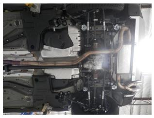
**Step 3.** Begin installation of your new MAGNAFLOW system by attaching the Inlet Pipe to the factory outlet using the supplied 2.25" clamp. Keep all clamps loose until final adjustment.
