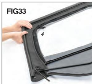
NOTE: the frame should fit in-between the hook and loop flaps, not between the zipper and the flaps.
