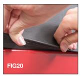
Step 11: Attach Side Curtains to Body Belt Rail
