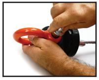
6. Thread shackle pin through rope loop, shackle eyelet, and shackle mount hole. Secure shackle as per normal operation.
