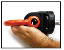
5. Align rope loop, shackle eyelet, and shackle mount hole.
