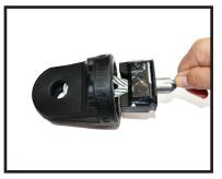
3. Apply two drops of lubricant to insert and spread evenly. Slip rope loop and insert into shackle mount cavity.
