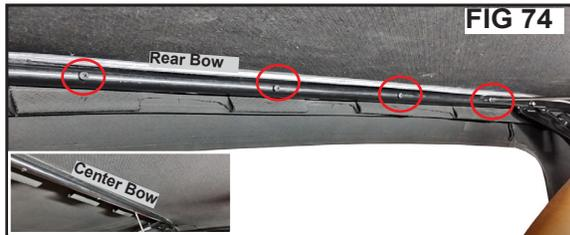
In the rear and center bow there are 4 screws installed into the bows. Remove the screws with a phillips head screw driver and set aside (Fig 74). Make sure the Soft top is centered on the rear bow
