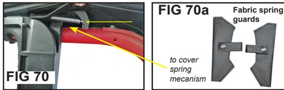
Locate the Cable spring hanging out of the soft top behind the rear seat next to the rear vertical door surrounds. With the front header tension released, attach the spring to the bracket shown in Fig.70 Make sure to hook the spring to the **top/first hole**. (the lower you hook the spring the more tension it will be when you fold down the header). **Keep the Front Header Folded Back.**
