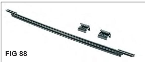
Locate the Tailgate bar and brackets (FIG 88). Locate the driver's side bracket. With the lip to the outside of the vehicle, line up the bracket with the slot in the body tub, hook the rear portion of the bracket to the body tub and roll the bracket forward until it click
