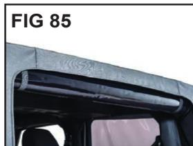
These straps can be used to secure your rear window when rolled up.
