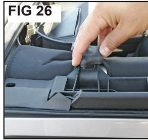
Line up the door surround “C” attachment holes with the vertical holes in the roll bar. Slip the front long knob through the hole in the front door surround (FIG25). Tighten the knob securing the front door surround (Fig 26).
