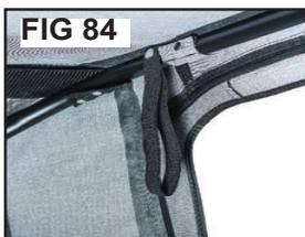
Locate the 2 elastic straps (Fig.83). Snap the elastic window roll straps on the rear bow above the rear win-
