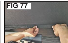
Go inside the vehicle, locate the front bow see fig 75, and the hook and loop flaps sewn into the top deck and secure. (FIG's 76 & 77).
