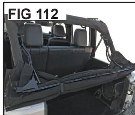
Unlatch the quick release knobs of the rear door surround bow bracket to the center bow and fold back the rear bow assembly just inside the rear tailgate bar as shown in fig's 106,107 & 108.
