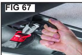
Drape the top fabric over the cab, as shown in fig 66. Unlatch the two front latches (Fig 67). With the help of a friend, lift up the Front header and fold it back until it seats on the top of your soft top.
