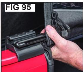
Tuck the flaps under the window zippers into the retainers to secure the rear window. See FIGs 96 & 97.
