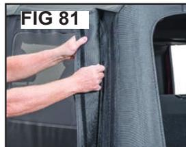
Roll the bottom of the quarter window into the retainer channel on the vehicle and then close the quarter window zipper the rest of the way.
