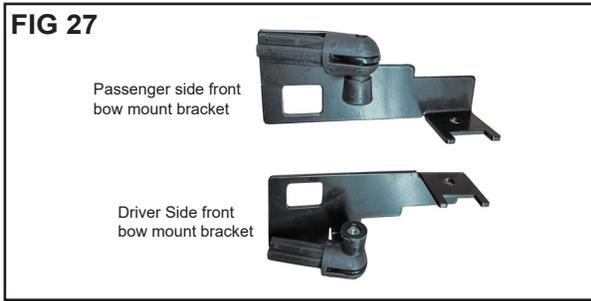
Locate the two front bow mount brackets as called out in FIG 27. The front bow mount brackets will be installed using the door surround short knobs that are included in the hardware pack. As circled in Fig 28, the oval mount is located towards the center of the vehicle. Take the drivers side front bow mount bracket and place the rectangle cutout over the oval mount as shown in Fig 29.
