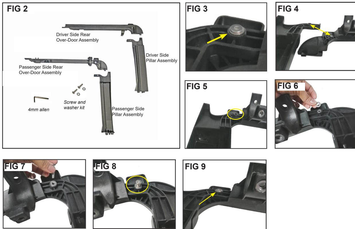
Locate the driver's side rear over door assembly and the driver's side Pillar assembly shown in FIG2
