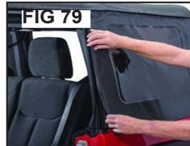
Attach the front of the quarter windows along the front edge of the vertical door surround by rolling the plastic into the slot on the door surround.
