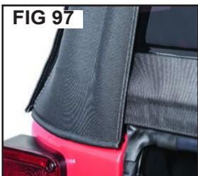
Tuck the flaps under the window zippers into the retainers to secure the rear window. See FIGs 96 & 97.
