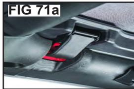
With the cable spring installed, use two people and simultaneously fold the header forward. Use the front header latches to secure the front of the top to the windshield. See FIG's 71-71a.
