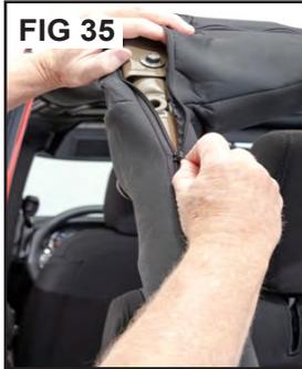
On the rear roll bar, un-hook the roll bar padding Velcro at the top of the roll bar and unzip the padding (Fig 35) which will expose the two factory mounting points on the inside of the roll bar. Place the roll bar mounting bracket over the holes and using the enclosed mounting bolts (T-30 Torx bolts) hand tighten the bracket in place (Figs 36 & 37).
