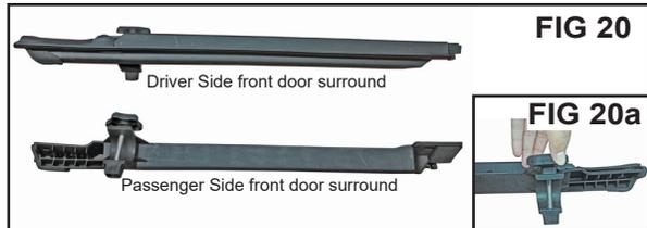
Locate the driver's side front door surround (Fig 20) and remove the knobs and set aside (Fig 20a). You will find an installed foam on the rear end. Line up the rear end with the front of the rear door surround as shown in FIG 21. Make sure the Door seals are not caught under the door surrounds. (See FIG22)
