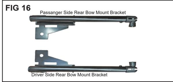
Locate the two rear bow mount brackets shown in Fig 16. Locate the Driver side rear bow mount bracket with the flat steel tab facing down and place the bracket over the door surround hole with the quick release knob facing in
