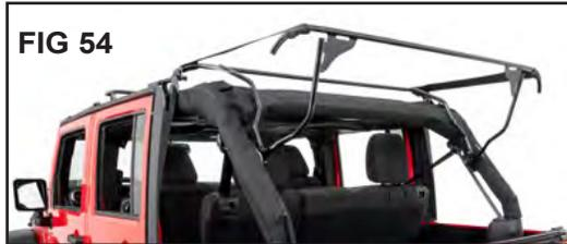
Once the bows are mounted to the roll bar mounts, lift the bow assembly up rotating it towards the top of the vehicle (Fig 50). You will be attaching the center bow to the rear door surround bow mount bracket you previously installed (Fig 51). Line the top bow tab to the bow mount quick release bracket and install the top bow to the mount by pulling the quick release knob out and you hear a “click” (Figs 52, 53 & 54). The rear bow system is now installed.
