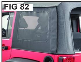
**NOTE:** You may have to loosen the side quarter window zippers and release the hook and loop when installing the rear window in step 16. This will make the Rear window install easier
