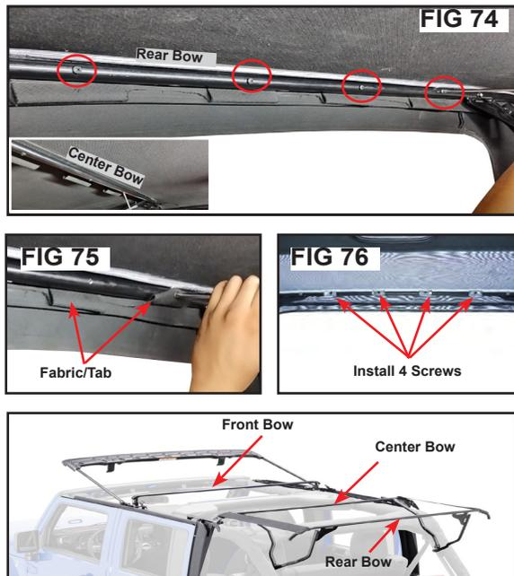
In the rear and center bow there are 4 screws installed into the bows. Remove the screws with a phillips head screw driver and set aside (Fig 74). Make sure the Soft top is centered on the rear bow
